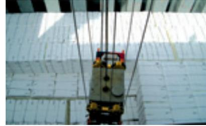
Howe Sound's shipping crew makes sure that the hold is tightly filled (with no voids), alternating the loading pattern so that there are no chimneys or stacks that might make the load unstable.
